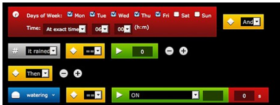
Fig. 11. Two scenarios defined using Fibaro (fibaro.com) platforms. The screen-shots show how different types of context triggered can be defined by combining sensors, actuators and predefined parameters.
