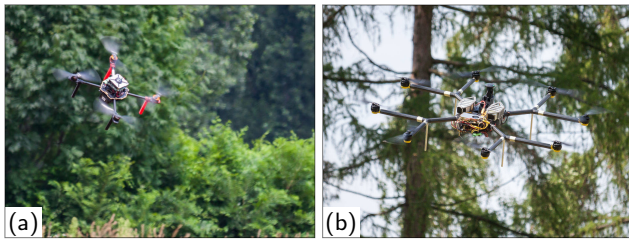
Figure 15: Novel control approaches can be tested on a real hardware. Off-the-shelf platforms such as (a) Tarot 650, and also (b) custom-built airframes, can be equipped with the proposed system.
