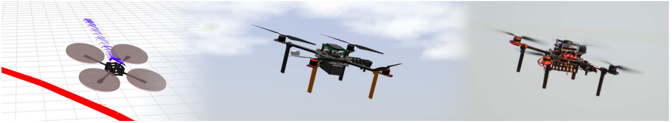
Figure 6: The Tarot 650 UAV platform is modeled with high fidelity within the simulation platform provided here.
