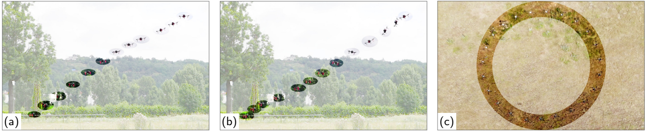
Figure 11: Photo collage of a UAV performing aggressive testing maneuvers. Figures (a) and (b) depict the UAV performing the 3D step reference, as showcased in Fig. 8. Figure (c) shows a top-down view of the circular trajectory, showcased in Fig. 10 and in Fig. 9. Go to http://mrs.felk.cvut.cz/mrs-uav-system for video material from the experiments.
