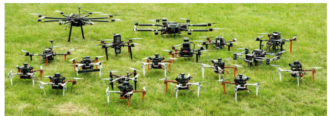
Figure 1: Multirotor UAV platforms equipped for various scenarios carried out by the system presented here.
