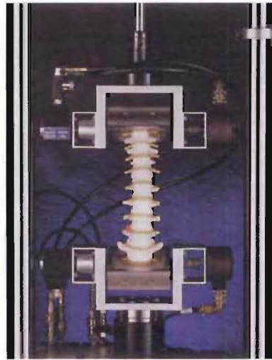
Figure 7.2 Flexion/extension and axial twisting module for a MTS machine.
