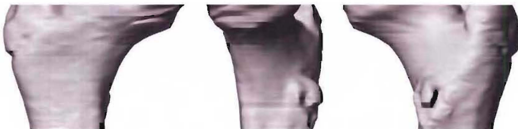
Figure 9.24 Lofted model of a partial femoral head developed from IGES curves.
