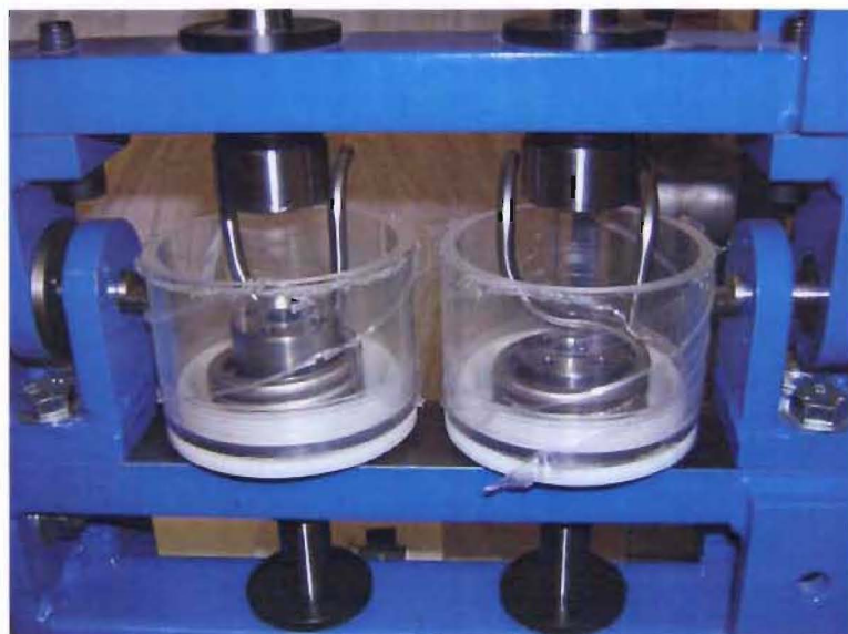
Figure 7.6 Single-axis test rig constraint mechanisms, fluid vessels and heating coils.
