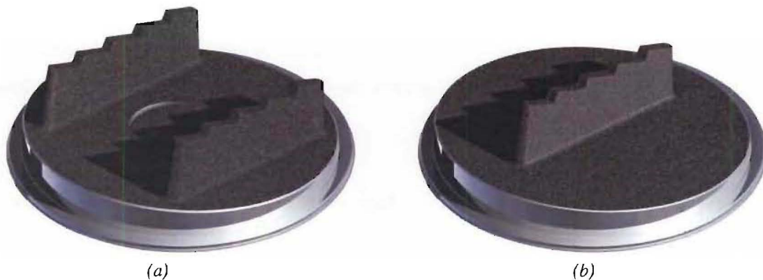
Figure 6.30 Rendered of implant endplates showing fixation features.
