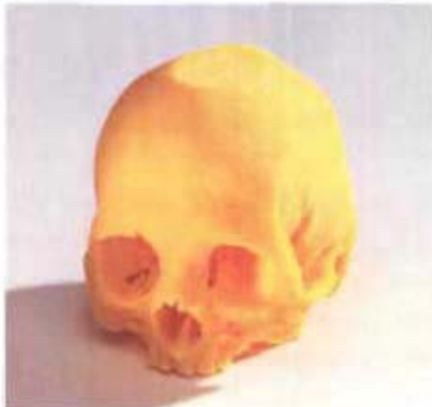
Figure 9.19 Human skull model created using three dimensional printing.
