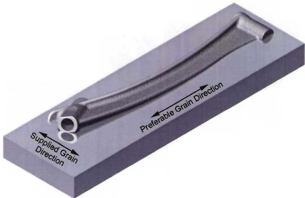
Figure 10.20 Endoprosthesis body, supplied and preferable grain directions.
