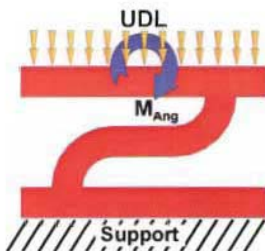
Figure A5.1 Schematic showing the loads applied to the Z-Spring concept.
