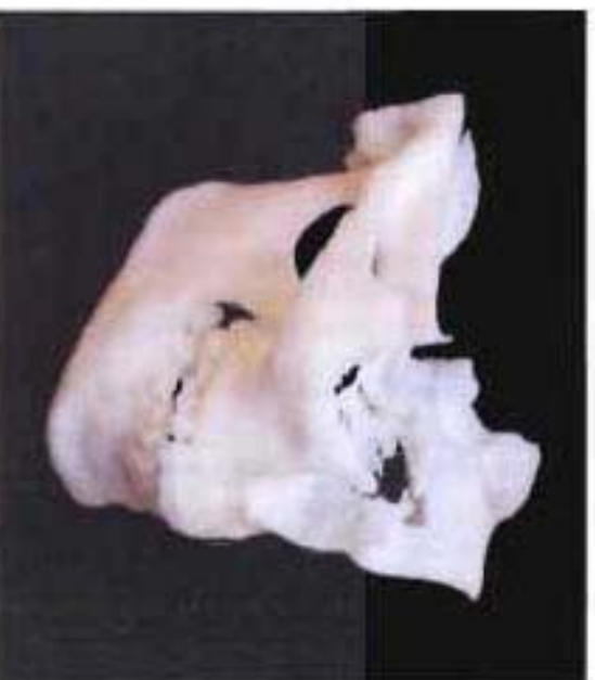
Figure 9.18 Fusion deposition model of a maxilla and mandible.
