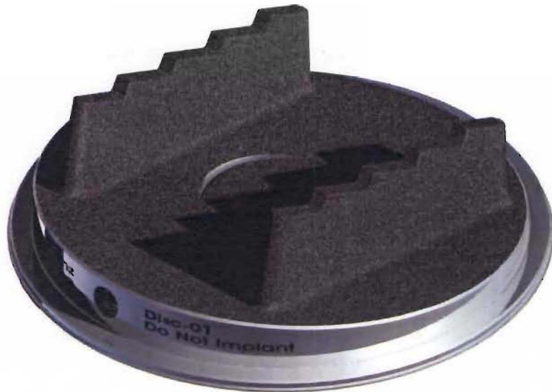
Figure 6.38 Example of laser engraving on the outer face of the top endplate. The engraving is shown positioned either side of the insertion/retraction tooling hole.
