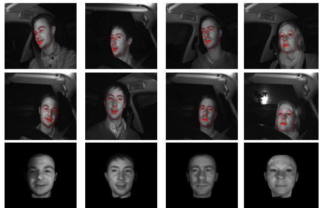
Fig. 3: Examples of face frontalization process [34] using facial landmarks. A simulated frontal view (bottom row) is generated from two side cameras (top and middle rows).
