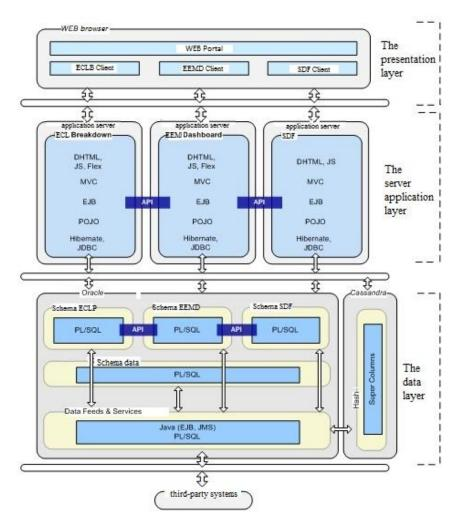
Fig. 3. - Fragment of the intellectual analysis system architecture
