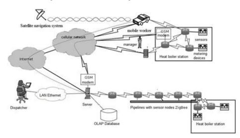
Fig. 2. - The wireless network segment for data collection of heating supply system
