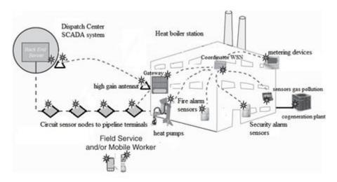
Fig. 1. - Sensor network cluster for heating points
