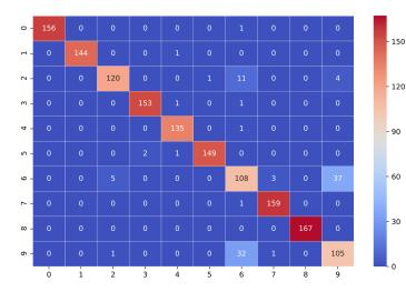
Figure 8: Confusion matrix of the neural network classifier to detect ten different *Arduino* programs which are labelled from 0 to 9.
