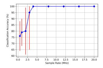
Figure 9: The effect of EM trace sample rate to the signal classification accuracy when used with 4 class classifier to identify four different *Arduino* programs.
