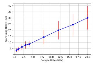
Figure 10: The variation of EM data processing overhead against sampling rate when used with 4 class classifier to identify four different *Arduino* programs.
