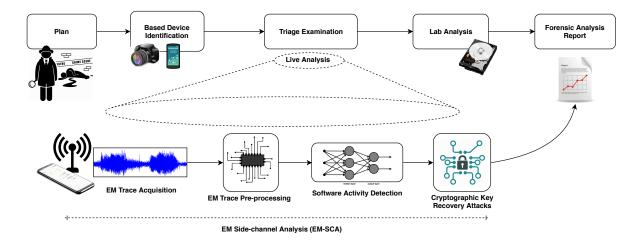
Figure 11: Integration of EM-SCA techniques into the standard digital evidence acquisition workflow (Adapted from Du et al. [35]).
