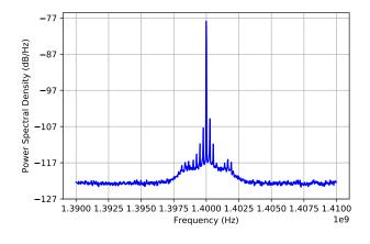
Figure 2: Power spectral density (PSD) of the Raspberry Pi device as observed around the clock frequency. A sampling duration of 0.01 seconds was used to capture EM signals for this work.
