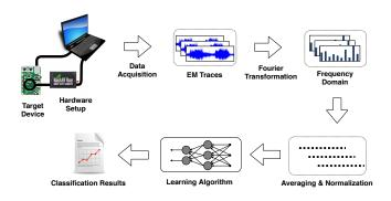
Figure 4: The EM trace acquisition and preprocessing stages in order to classify cryptographic activities using a machine learning model.
