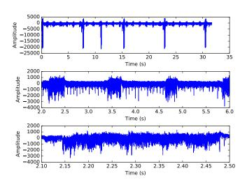
Figure 3: Waveform of the AM demodulated signal at the CPU clock frequency of Raspberry Pi. The AM modulated signal represents the AES encryption performed on the device. Sudden higher peaks are an external interference signal coming from an unknown source.
