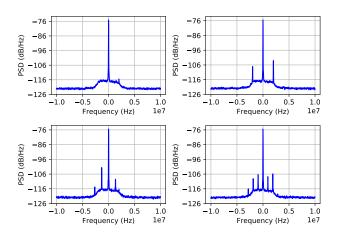
Figure 7: Power spectral density (PSD) of the EM emission from four different *Arduino* programs which were used for classification.
