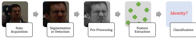
Figure 1: General pipeline of a face recognition system. From a pattern recognition perspective, the most significant modules of a biometric system are the sensor module, the segmentation module; the feature extraction module; and the classification or decision-making module.
