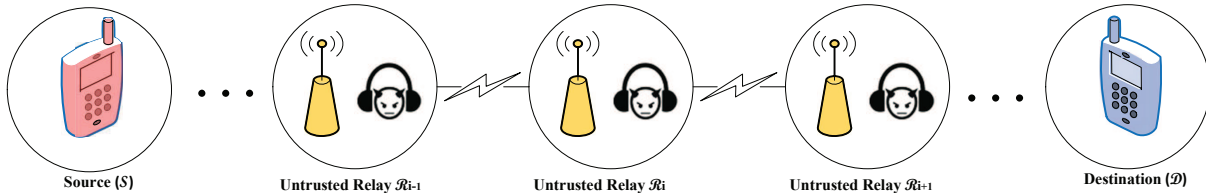
Fig. 1. System model of secure multi-hop untrusted relaying.
