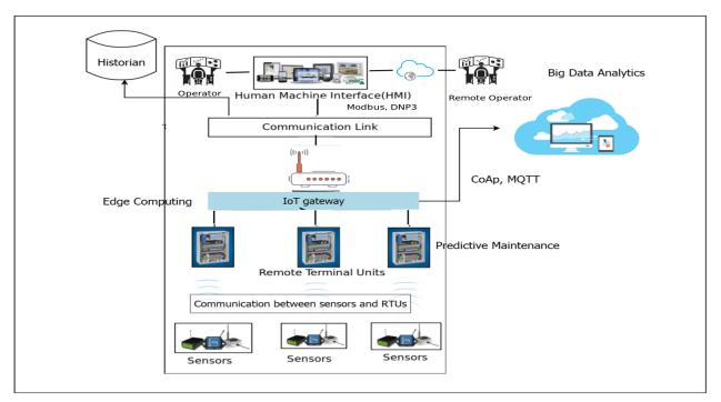
Figure 8: Fourth generation SCADA
