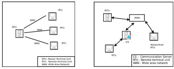
Figure 5: Monolithic SCADA system Architecture
