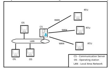
Figure 7: Distributed SCADA system Architecture
