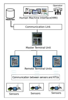
Figure 4: Interrelation of SCADA system components (inspired by [7])
