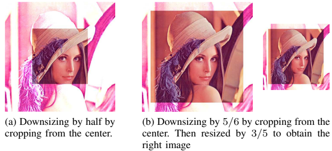
Fig. 4: The effect of cropping on field of view: The sensor captures the full resolution image. The saturated regions (borders) are discarded and the centers are the final images.
