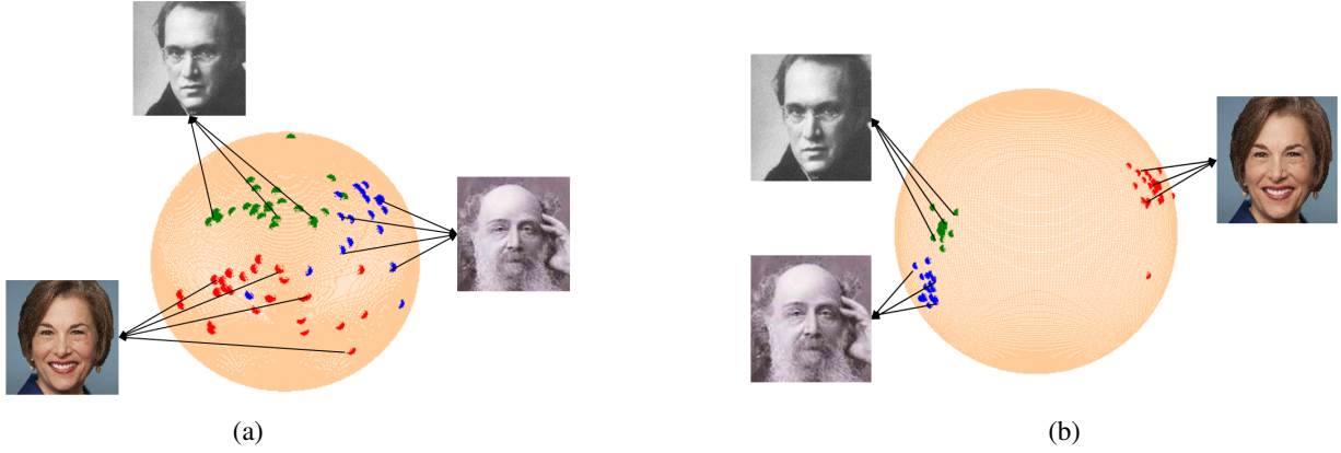
Fig. 4. Three-dimensional normalized features for three different identities, obtained from (a) network trained with Softmax Loss. (b) network trained with Crystal Loss. The intra-class cosine distance reduces while the inter-class cosine distance increases by using the Crystal Loss.
