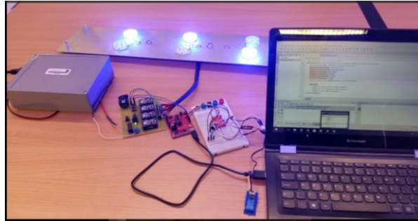
Fig. 5: Functional Integrated System Hardware Showing all the Devices Used in the Design
