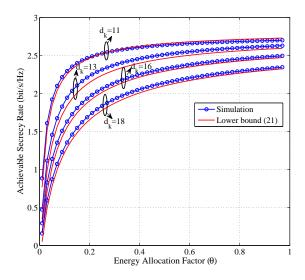
Fig. 4. User's achievable secrecy rate versus the fraction of energy allocated to pilot training by the user. The users and eavesdropper distance from the BS are  $d_k = [11, 13, 16, 18]$ ,  $d_w = 15$ , respectively and  $\rho_k = 0.4$ .
