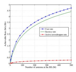
Fig. 7. Achievable Rates versus the number of antennas at the BS. The user and eavesdropper distances from the BS are  $d_k$  = 13 and  $d_w$  = 15.  $\rho_k$  = 0.4 and  $\theta$  = 0.7
