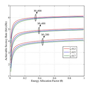
Fig. 6. Average achievable secrecy rate versus the fraction of energy allocated to pilot training by the user. The user and active eavesdropper distances from the BS are  $d_k$  = 13 and  $d_w$  = 15, respectively. User power splitting ratio and eavesdropper power splitting ratio are set  $\rho_k$  = 0.4 and  $\zeta$  = [0.2 0.5 0.7] for the number of antennas at BS M = [200 400 800].
