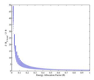
Fig. 9. Positivity of derivative function of the secrecy rate lower bound according to harvested energy allocation factor  $(\theta)$ . The derivative function of secrecy rate lower bound is plotted for various locations of the users and the active eavesdropper.  $d_k \sim \mathcal{U}[10, 20]$  (meters) and  $d_w \sim \mathcal{U}[10, 20]$  (meters).
