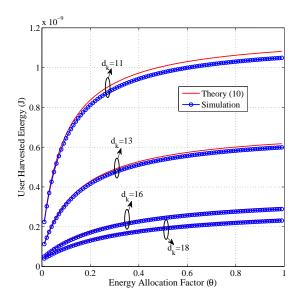
Fig. 3. Average user's harvested energy versus the fraction of energy allocated to pilot training by the user. The users and eavesdropper distance from the BS are  $d_k = [11, 13, 16, 18]$ ,  $d_w = 15$ , respectively and  $\rho_k = 0.4$ .
