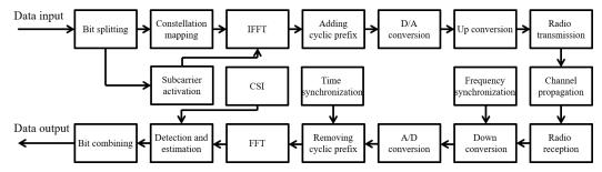
Fig. 1: System diagram of a typical DF relay assisted OFDM-IM system.
