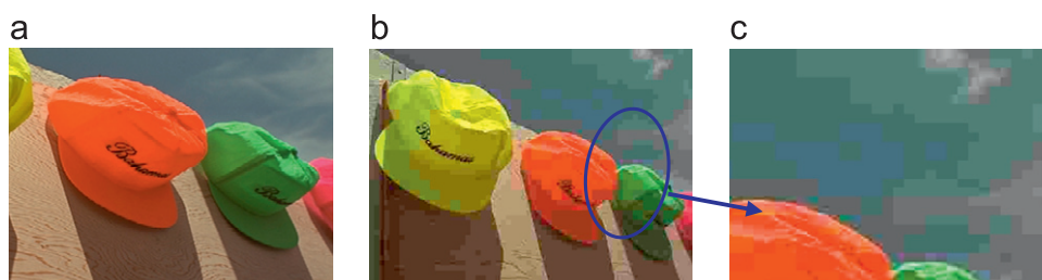
Fig. 1. JPEG compression distortions: (a) original image, (b) JPEG blocking effect, (c) zoomed version of image (b).
