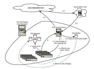
Figure 1. High-level diagram of caching-proxy operation. The same steps happen for both proxy implementations.
