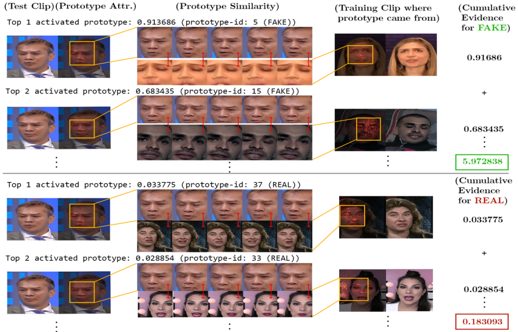
Figure 3: The reasoning process of the DPNet. The prediction for each class is based on the evidence between the dynamics of the input and a small set of dynamic prototypes. Best view as GIFs (See C).
