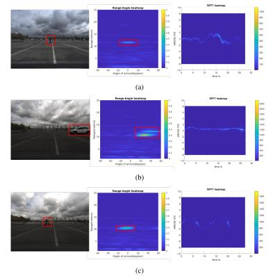
Fig. 8: (a) Single moving pedestrian (b) Single moving car (c) Single moving cyclist. For each row, there are camera image (left), RA heatmap (center), and STFT heatmap (right)
