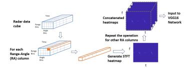
Fig. 10: STFT processing for radar data cube
