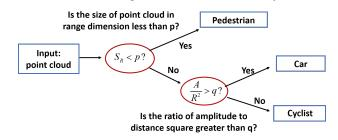
Fig. 11: Decision tree baseline, where A is the averaged amplitude of point cloud, R is the distance to radar,  $S_R$  is the point cloud size in range, i.e. the number of points in range, and p, q are threshold scalars
