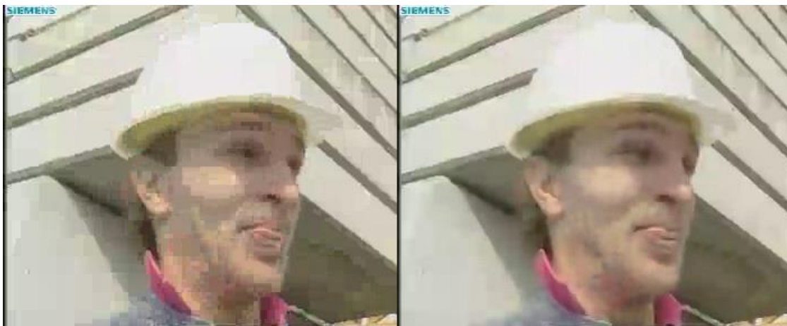
Figure 5 - Example of deblocking filter performance: without (left) and with (right) deblocking filter [7].
