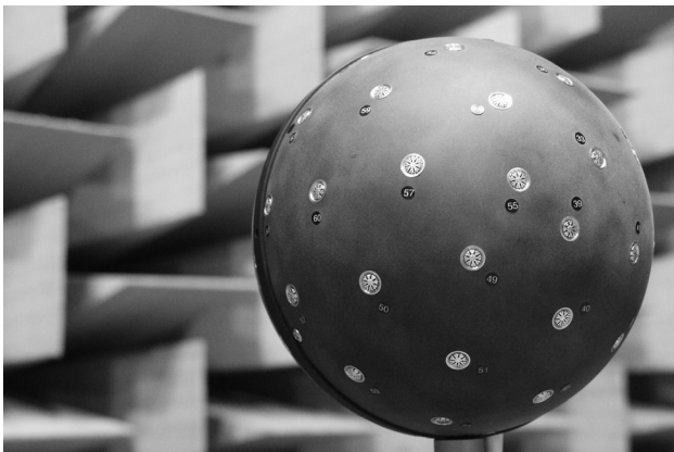
FIG. 5. Sixty-four-channels rigid spherical microphone array.
