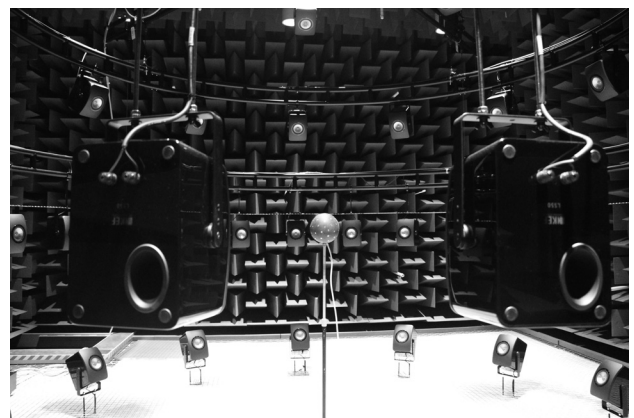
FIG. 8. Sixty-four-channel loudspeaker array (Audio Visual Immersion Lab, AVIL, DTU).
