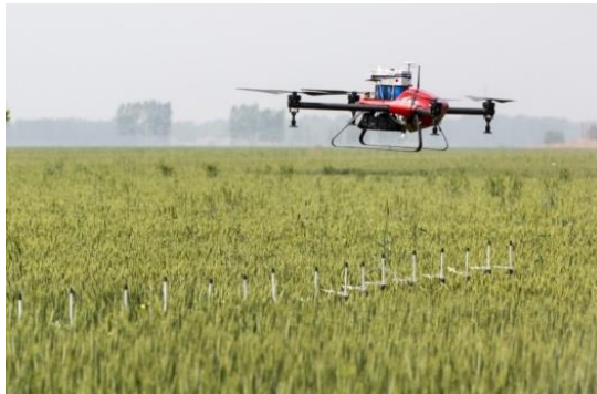
a. P-20 UAV spraying on wheat by XAIRCRAFT Co., LTD
