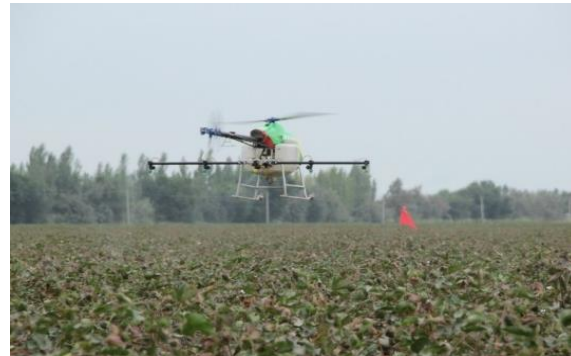
b. HY-B-15L UAV spraying on cotton by Shenzhen Hi-tech New Agriculture Technologies Co., LTD
