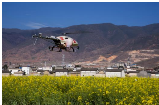
c. 3WQF125-16 UAV spraying on cole by Quanfeng Aviation Plant Protection Technology Co., LTD
