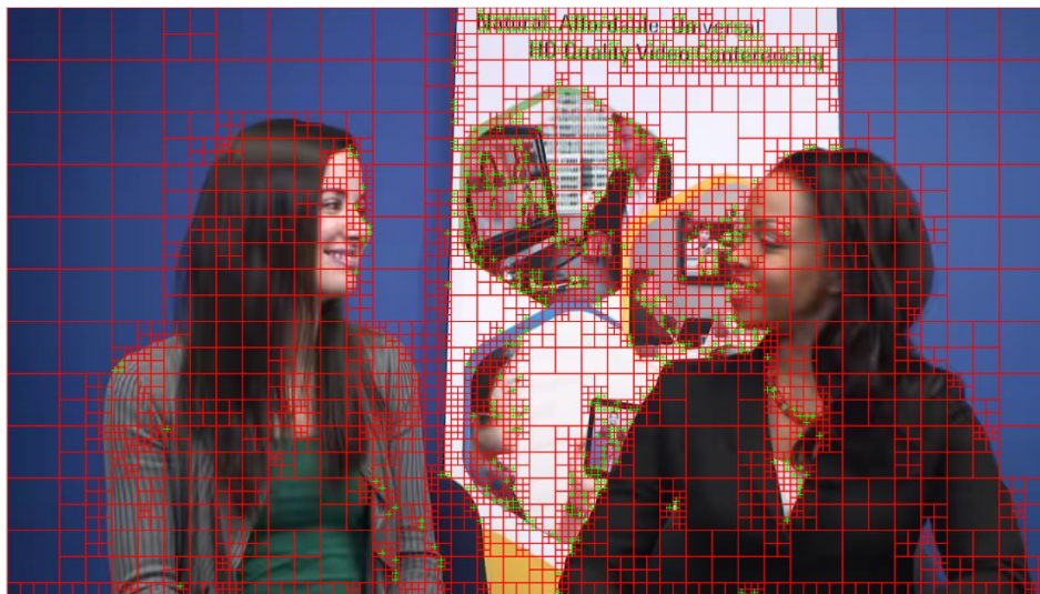
Figure 1. Coding Unit (CU) partitioning structure for a typical intra-predicted frame in “Kristen and Sara” sequence.
