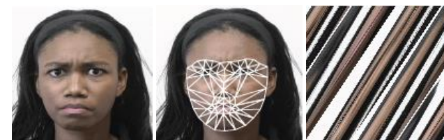
Fig.2. Semantic approaches such as using AAM [18]~[25] for facial emotion estimation cannot be applied in the scrambled domain.
