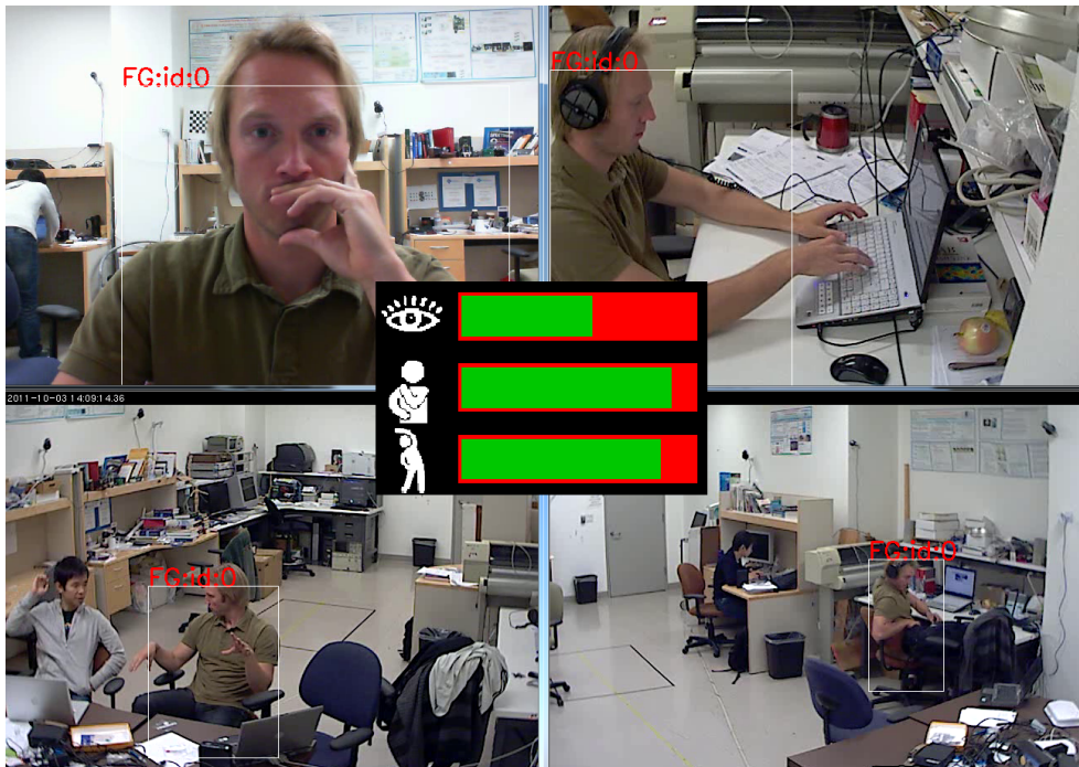
Figure 9.1: Personalized Ergonomics: A multi-camera system monitors worker's daily activities around the office. Based on context-aware observations measures on attention, posture and mobility are computed. The personal data is accumulated over time based on which guidelines are personalized and feedback is given to the user.
