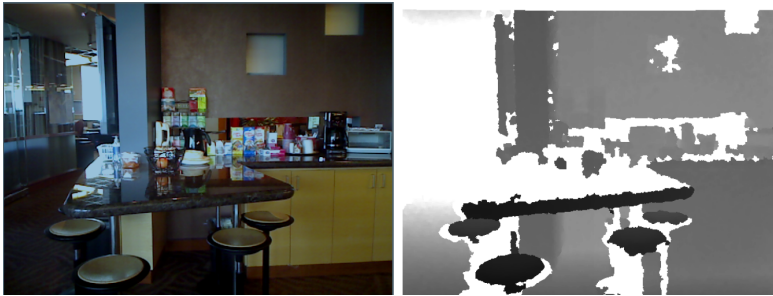
Figure 3.8: Left) RGB image, and right) depth information captured by an RGB-D camera. Systems of 2011 can capture images up to 640 \times 480 pixels resolution at 30 frames per second. White pixels on the right image are without depth value, mostly due to occlusions, maximum distance, and surface angle and material. With permission from [48].
