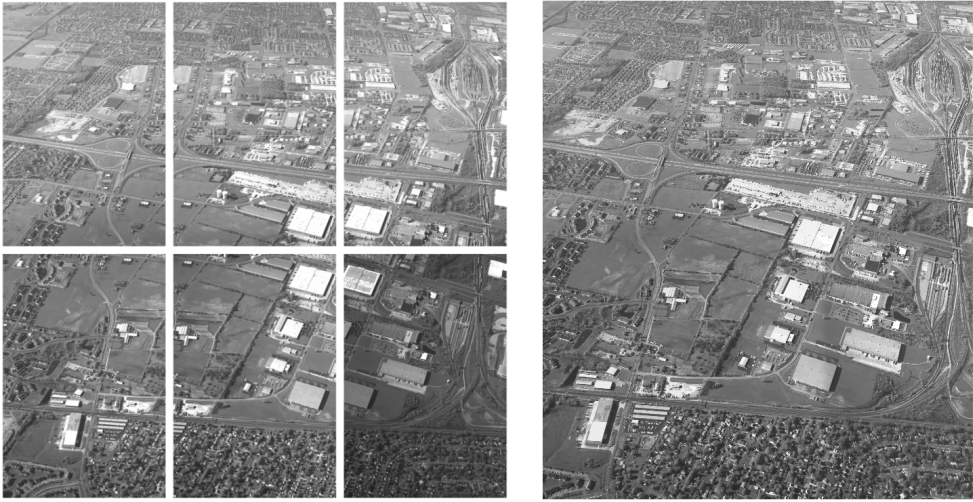
Figure 3.16: Image Mosaic: left) an array of cameras captures part of a scenery, right) a single virtual image covering entire area is created for scene analysis. With permission from [67].
