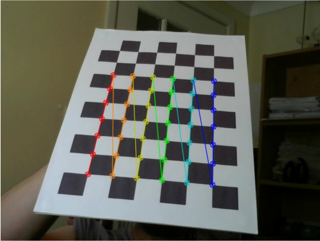
Figure 7.7: A camera calibration board.
