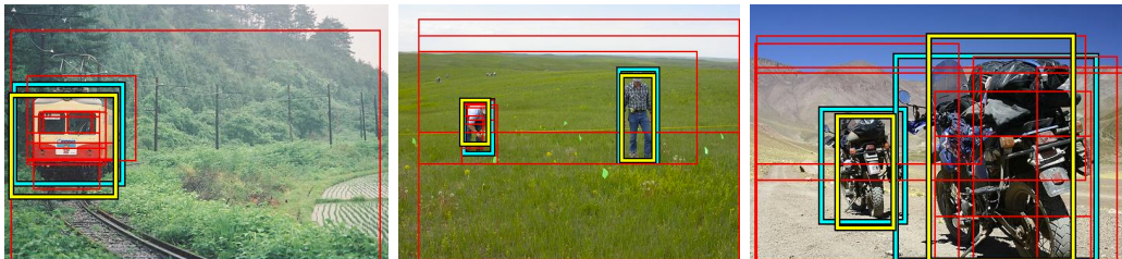
Figure 1.3: A class-generic object detector [Alexe et al., 2010] that discards non-object sliding windows in the image.
