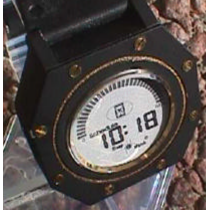
Figure 5-1. The Sleep Watch Actigraph (SWA) showing fuel-gauge-type current performance capacity read-out.
