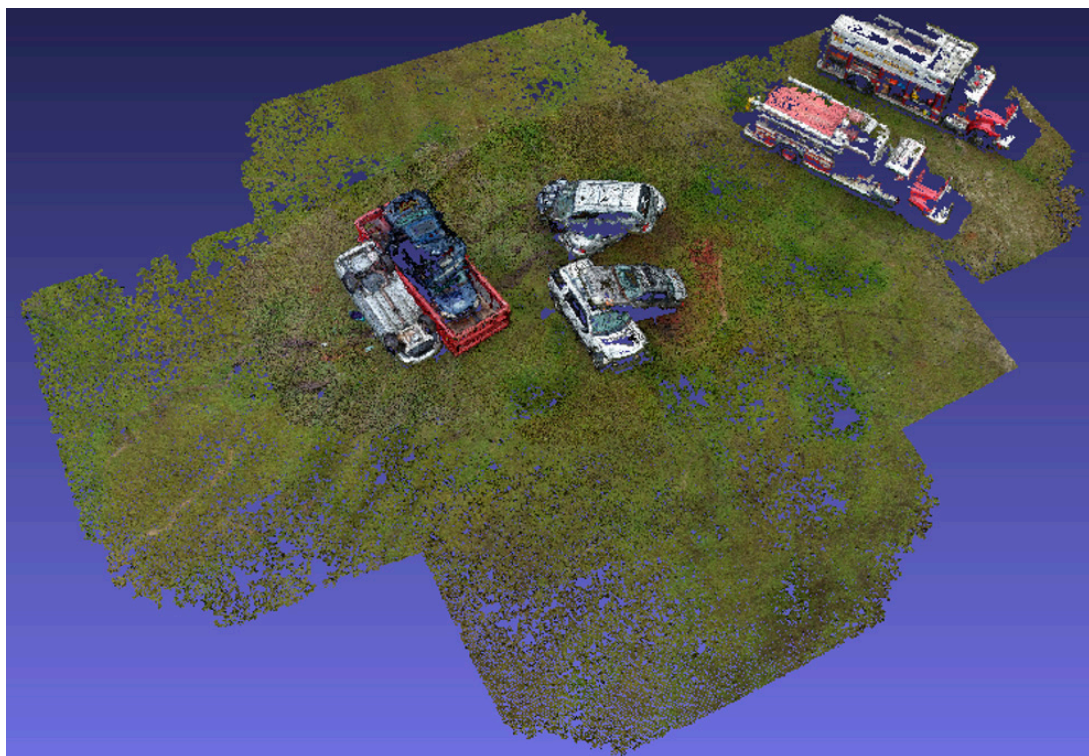
Figure 14. The sparse point-cloud model for the forensic dataset, and constructed by the ISFM system with the RTFT feature tracking method.
