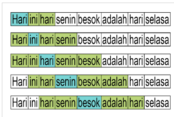
Figure 1 Illustration of sliding window in Word2Vec
