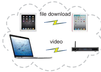
Figure 6.2: QoS based autonomic self-optimization system setup with four devices on the same ad-hoc network, arranged in two transmitter/receiver pairs.
