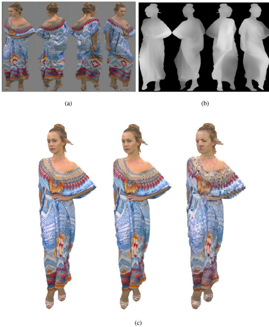
Fig. 4. Projected (a) texture and (b) geometry images for (c) original point cloud (left), as well as decoded point clouds at 13 MBit/s for the proposed solution (middle) and reference technology [2] (right).
