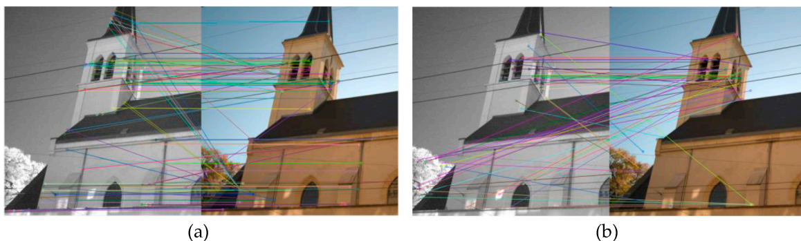
Figure 1. (a) Infrared image-matching results of scale-invariant feature transform (SIFT); (b) Visible image-matching results of speeded-up robust features (SURF) algorithms.
