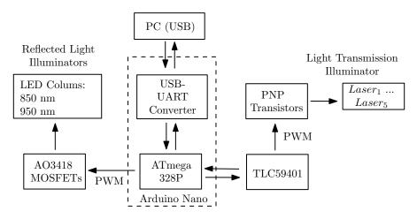
Figure 5. Schematic structure of the illumination control board.
