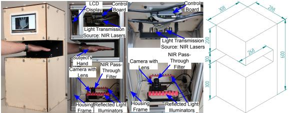
**Figure 2.** Contactless finger and hand vein capturing device, from left to right: device in use during acquisition, side view with annotated parts, top side view and bottom side detail view, housing including dimensions.
