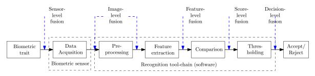
Figure 7. Biometric recognition tool-chain and different levels of biometric fusion.
