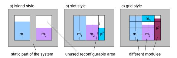
**Figure 2.1.:** The different configuration styles for designing partial reconfigurable systems. On the a) *island style*, only one module can exclusively be loaded in one area at the same time. The b) *slot* and c) *grid style* can host multiple modules with different shapes. Taken from [21].
