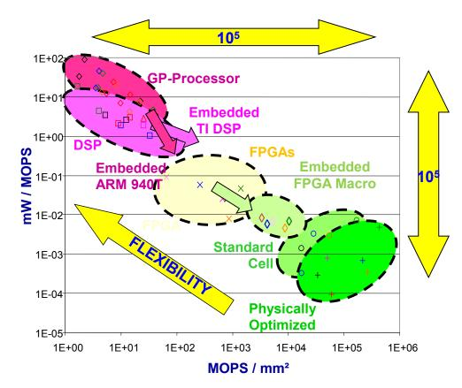
Figure 1.2.: Energy and area efficiency of different implementations of sample applications. All entries are properly scaled to 130 nm CMOS technology. Furthermore, the increasing flexibility is depicted. Taken from [34].
