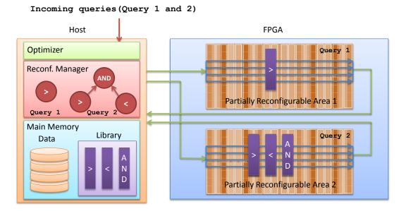
**Figure 3.1.:** An overview of the query acceleration system: Each incoming query is analyzed by the Reconfiguration Manager and corresponding modules of the generated query execution plan are loaded subsequently onto the FPGA. On the right, two partially reconfigurable areas are depicted which even allow the simultaneous processing of two (partial) queries in parallel. Taken from [J1\*].
