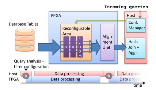
**Figure 3.2.:** Overview of the new architecture for hardware-accelerated query processing (above). First, an incoming query is analyzed and a filter chain configured by parameter adaptation and, if necessary, by structure adaptation through partial dynamic reconfiguration. Afterwards, the data is streamed through the filter chain and in the meanwhile, the already filtered data is processed by the software implemented hash join (see timing diagram below). Taken from [C5\*].
