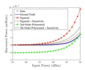
Fig. 2. Harvested power (in milliWatt) versus input power (in dBm) for the harvester proposed in [6] using nonlinear harvested power function  $p_n(\cdot)$ , n=3,4,5,6, as well as for the ground truth model in Eq. (4). Input power range within [-45,-20] dBm.
