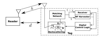
Fig. 1. Monostatic backscatter architecture consisting of a reader and a passive (i.e., battervless) RFID tag. Reader acts as carrier emitter, as well as receiver of tag reflected/backscattered information.
