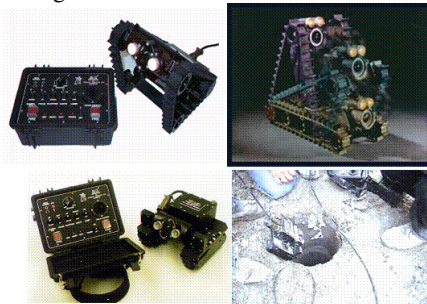
Figure 1: The Micro VGTV System by Inuktun with its control units
