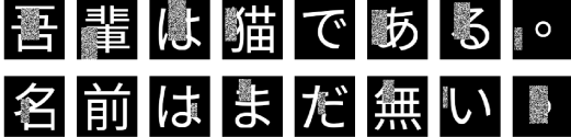
Fig. 2. Example of data augmentation on image domain (random erasing data augmentation [17]). Note that this is an example of an implementation on this experiment and augmentation is not limited to this method.
