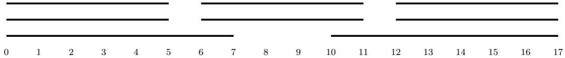
Figure 1: An instance of interval scheduling maximizing minimum coverage in which 8 intervals are given and k = 2 machines are available to execute them. Observe that in all solutions to this problem three disjoint intervals of length 5 need to be removed, leading to a solution that executes 5 jobs and the number of idle machines is never greater than 1. However, in the solutions to the classical interval scheduling with given machines problem, the two intervals of length 7 are removed both in the case when all intervals have the same profit, and in the case when the profit of an interval equals its length.
