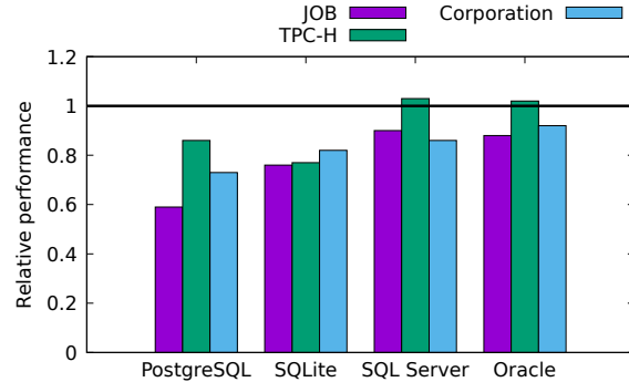
Figure 9: Relative query performance to plans created by the native optimizer (lower is better) for different workloads
