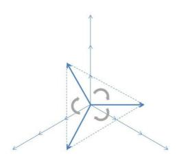
**Fig. 1.** A schematic showing the symmetric tetrahedron formed by the permutation of the coordinates of either the electric or the magnetic field components. Their common summand must then lie on the height of the tetrahedron drawn from the origin of the coordinate system.
