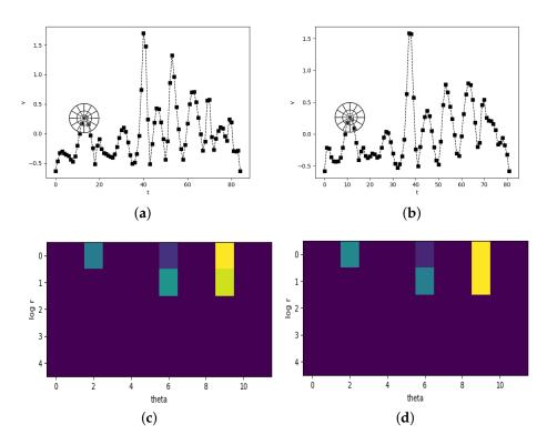
**Figure 4.** SC-DTW. ( $\mathbf{a}$ , $\mathbf{b}$ ) Time series of total velocity v from two signatures and a pair of corresponding points found by shape context. ( $\mathbf{c}$ , $\mathbf{d}$ ) show the shape context histograms of the points marked in ( $\mathbf{a}$ , $\mathbf{b}$ ), respectively.
