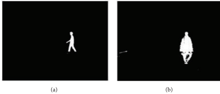
FIGURE 4: Threshold suppression. (a) Initial segmentation using Otsu threshold. (b) Segmentation by adding parameter c .
