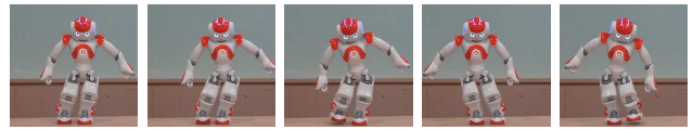
Fig. 4. Cautious walk: the robot makes high and slow steps, while looking at the ground.
