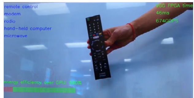
Fig. 10. Object recognition: A VGG network running on NovuMind's AI processor FPGA prototype performs real time object recognition. Upper left-hand corner lists the top-5 recognition results.
