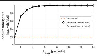
Fig. 2. Throughput in packets/slot versus maximum secret-key buffer size.
