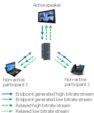
Figure 2.9: Logic of SFU based on Scalable Video Coding
