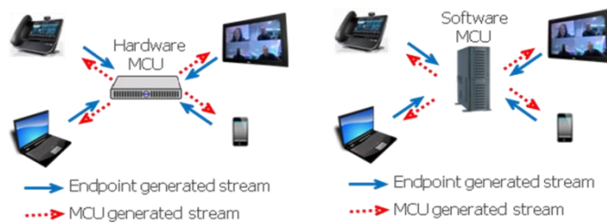
Figure 2.8: Logic of MCU
