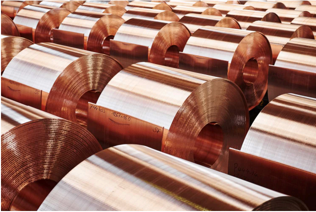
Fig. 6: Cast-rolled copper strips from Conti-M® (source: MKM)
