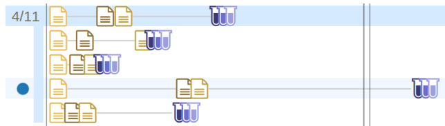
Figure 7: Example of an expanded variant which originally contains 11 traces in total and 4 of them match the current filter setting. A selected trace is indicated by the blue dot at the left of the trace.
