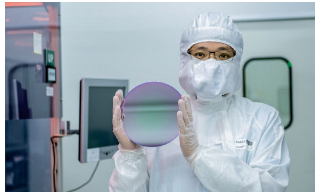
The first independently developed 8-in. radiation-hardened silicon-on-insulator (SOI) wafer, manufactured by SIMIT
