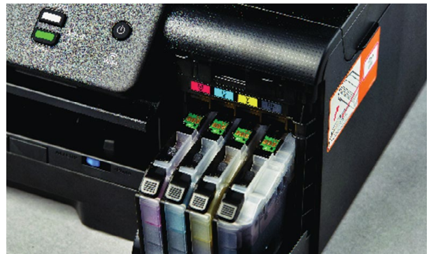
Mass-produced PCRAM chips used in printer ink cartridges
