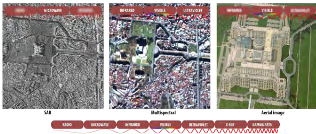
FIGURE 2. The House of Parliament, Bucharest: 3 different energy signatures measurements obtained using 3 different sensors: Sentinel 1 (left), Sentinel 2 (center), aerial (right).
