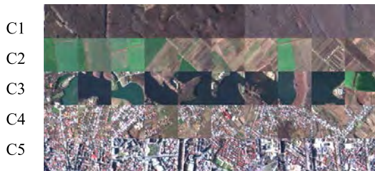
FIGURE 30. Samples form the training set used for the analysis of the Sentinel 2 image. The selected classes are: forest (C1), agriculture (C2), water (C3), sparse urban (C4), dense urban (C5).
