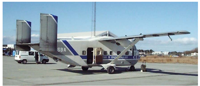
Figure 6. Skyvan with aft and nadir pointing EMIRAD antennas.
